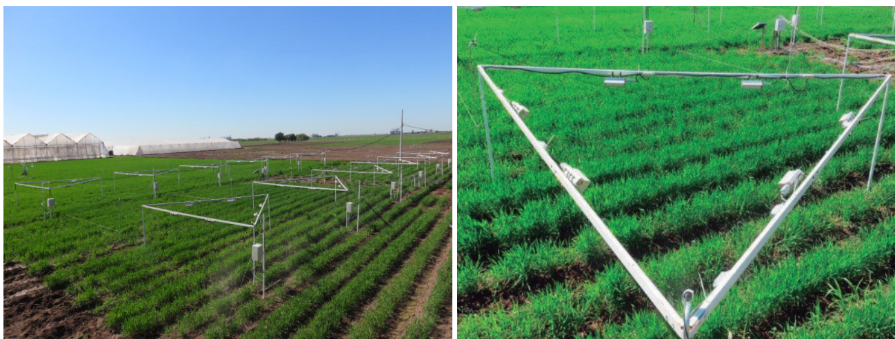
Figure 1. Top view of 12 repetitions of the triangular structure that was used to install the heat radiators, separated at a distance of 1.20 m from the canopy of the crop
