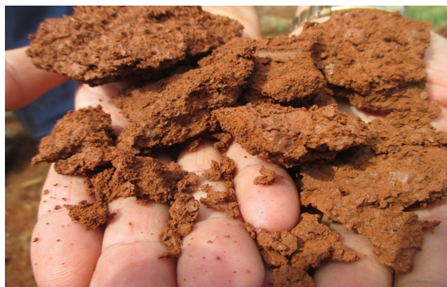
Figure 3. Horizontal angular block structure of the studied profile
